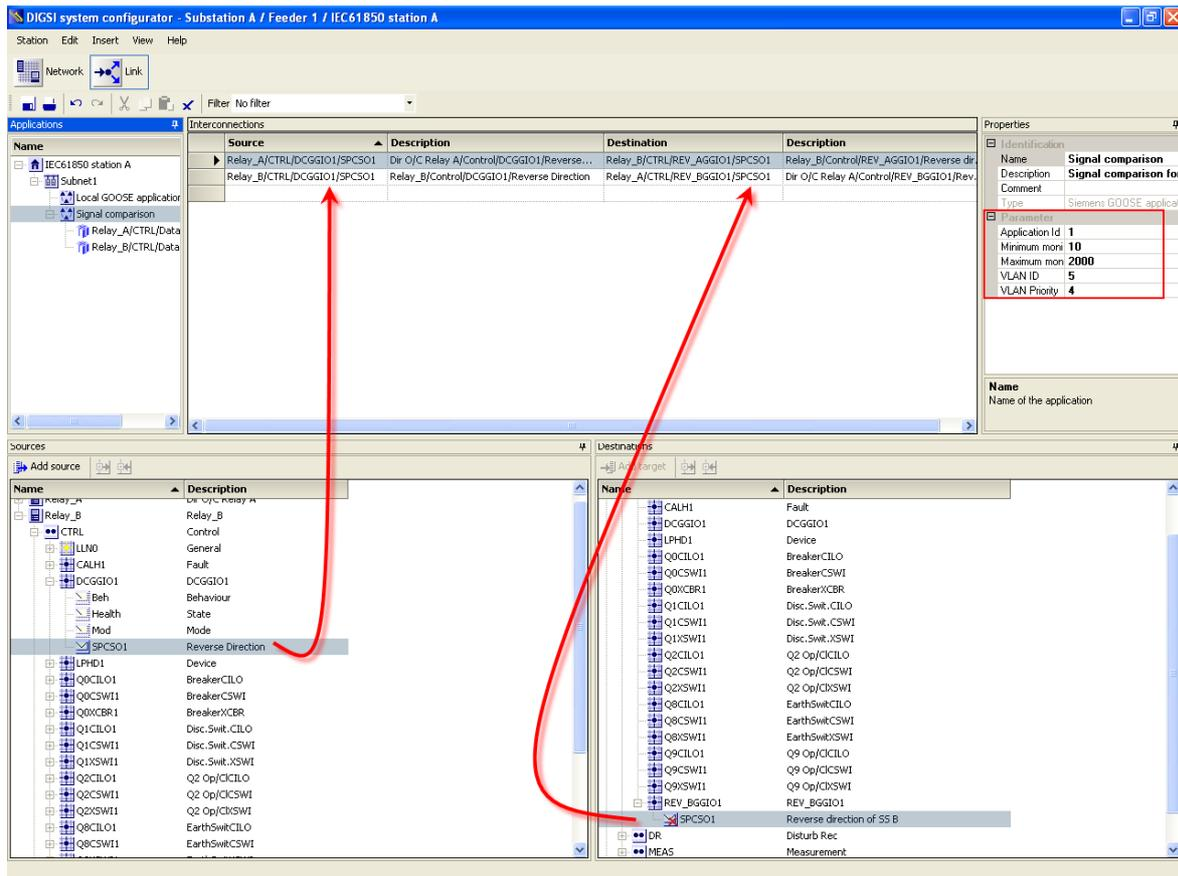
**Fig. 14: Configuration of GOOSE – messages for SS2SS – communication in substation A. The same engineering step must be done for B.**
