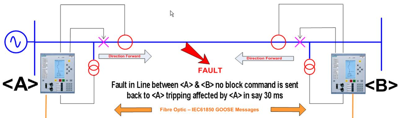
Figure 3: Reverse Block Principle across a line – Fault in line
