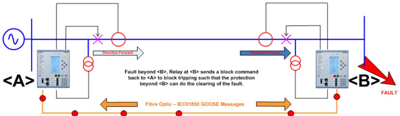
**Figure 3: Reverse Block Principle across a line – Fault outside line**
