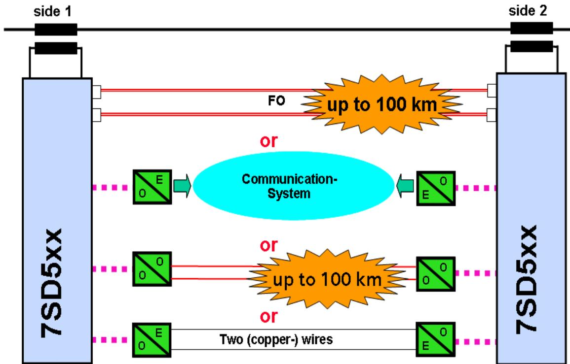
Figure 1: Existing setup for teleprotection communication with integrated digital serial interface.
